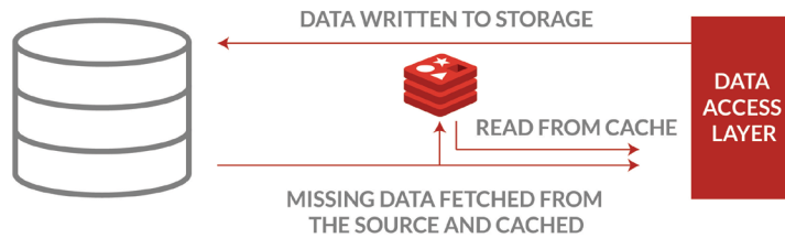
Figure 3. A simple look-aside cache architecture
