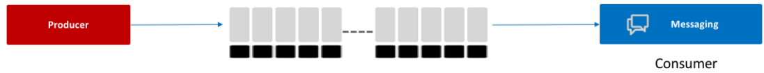
Figure 1.1. A simple application of Redis Streams with one producer and one consumer.
