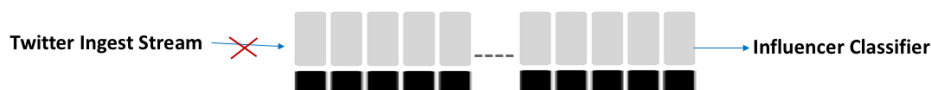
Figure 3.4. The consumer must wait for new data to arrive when the ingest stream is disconnected.
