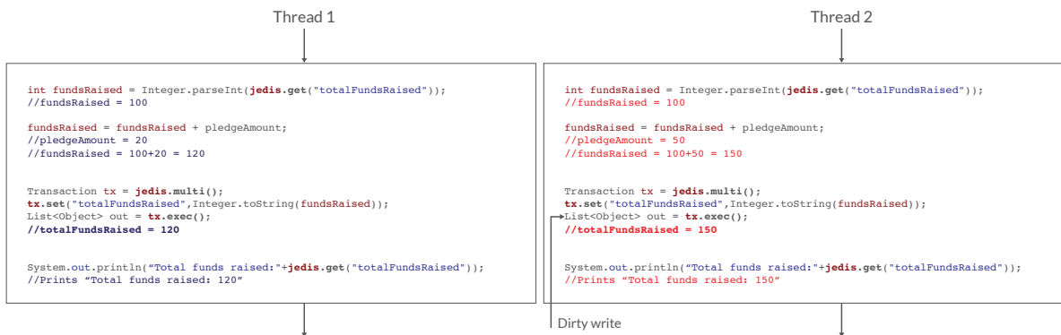
Figure 5. Two threads reading and writing to the same key. Thread 2 writes over the data written by Thread 1
