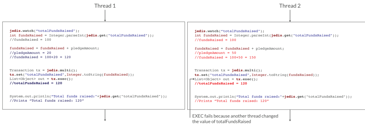
Figure 7. Two threads writing to the same key. WATCH command forces the second update to fail
